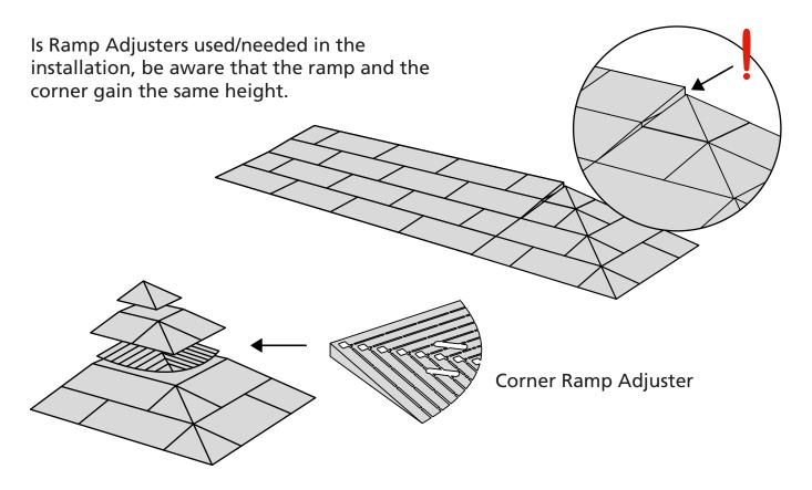
Corner Ramp Adjuster height adjustments:
